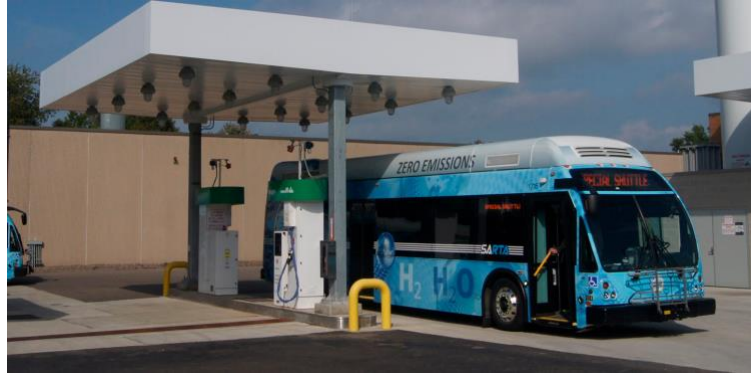
Fuel cell bus refueling at Stark Area Regional Transit Authority
